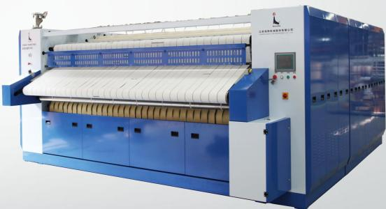
Designed with a high-efficiency serpentine layout, this advanced ironer maximizes heat transfer and fabric contact, enabling faster ironing speeds and flawless linen results—even with high-moisture loads. The multi-roll serpentine design increases surface exposure without increasing footprint, saving space while boosting throughput.
