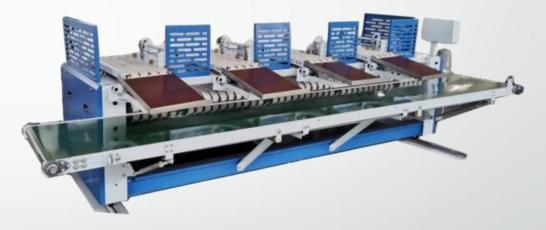
Fully automatic pillowcase folder ZDZT-3400 is designed to fold and accumulate pillowcases after ironing and can be used with various corresponding folding machines.
